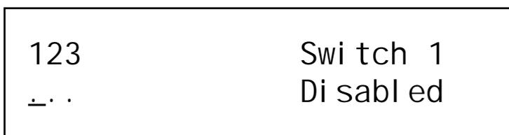
Page 4 in the Midi menu has a single parameter for each of the three pedal / switch jack sockets. This parameter determines whether pedal / switch MIDI data will be transmitted ( and passed on to the Part ). If the jack socket parameter is set to "Enabled" ( "o" ), then when the pedal / footswitch is moved, the appropriate MIDI data will be transmitted using the Part's own MIDI channel. This MIDI data will then be passed to the Part.
