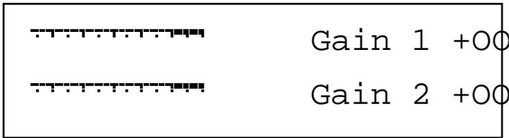
Inputs 1 & 2 can be monitored, and the sensitivity of the inputs can be adjusted using this page. Peak Program Meters show the level of both inputs. The levels of each of these signals can be adjusted from +60 dB gain to -8 dB attenuation using the upper and lower Data knobs. These parameters are memorised with the Global settings.
