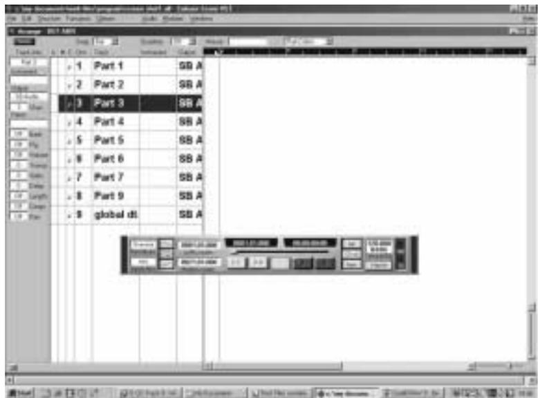
Similarly, to play or edit Part 3, first select (highlight) the sequencer track corresponding to Part 3 and then select Part 3 on the Supernova II Keyboard's front panel. Part 3 can now be edited, played or assigned its own Program using the Supernova II's front panel controls. The MIDI information transmitted by Part 3 is being re-routed back to the Supernova II Keyboard's MIDI channel for Part 3 (MIDI channel 3).
