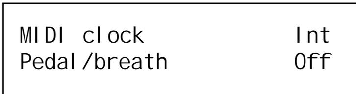
For example, if the "Pedal/breath" parameter in the Global menu was set to "MW", all data generated by the pedal would be passed on to the currently selected Program as if it were modulation wheel data (CC 1) taking into account all of the Wheel settings in the Program's modulation matrices.
