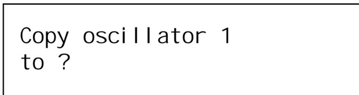
It is now a simple matter of pressing the destination ( the Oscillator that you wish to copy oscillator 1’s settings to ). i.e. Press Oscillator 2 button and the display shows:
