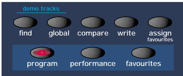
To select a specific number requires only 2 button presses - even if the number has 3 digits. For example to select Program 123, make sure the Supernova II keyboard is in Program Mode ( the Program button is lit ). Now simply press the '120' button followed by the '3' button in the Keypad section. The display shows:
