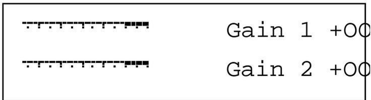
In this page meters are available showing the level of incoming signals on each of the 2 Inputs. The 2 Data knobs access "Gain" controls allowing -8dBm attenuation ( a signal of +8dbm will clip ) to +60dBm of boost or gain to the signal. When the meters reach the highest segment of the display, the signal is clipping. Set the "Gain" controls to get the loudest possible signal without clipping.
