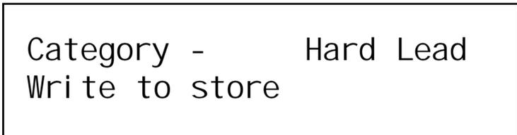
The Supernova II keyboard is asking for confirmation that you wish to write over the destination Program, replacing it with the newly edited sound. On the top line of the display, it can be seen that there is the category parameter. This is where you set the category of the Program so that the "Finder" mode can locate programs with the same category assigned. To adjust this parameter, use the higher Data knob. There are 20 different categories. Refer to page 47 for details on the categories.
